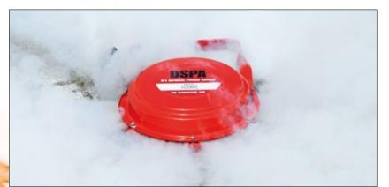
DSPA Aerosol was originally developed as an alternative to Halon. Unlike Halon, DSPA is environmentally friendly. The active substances of the DSPA Aerosol are solid micro particles that fill the compartment completely and attack the combustion process at a chemical level. As a result, the flames are instantly knocked down and the energy removed from the fire.
